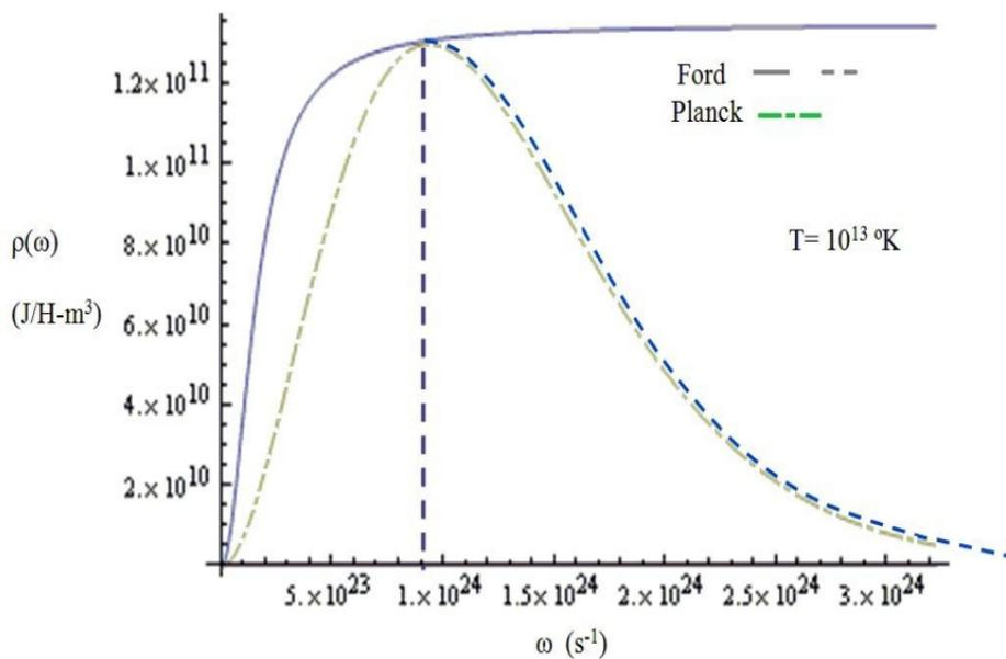
Figure 2: Density of radiation by using the Eliezer-Ford equation
