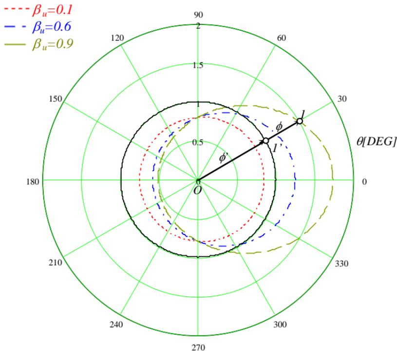
**Figure 3.** The relativistic diagram displaying in true magnitudes the scalar components of four vectors that transform like the time coordinates of the events generated by the moving bullets do.
