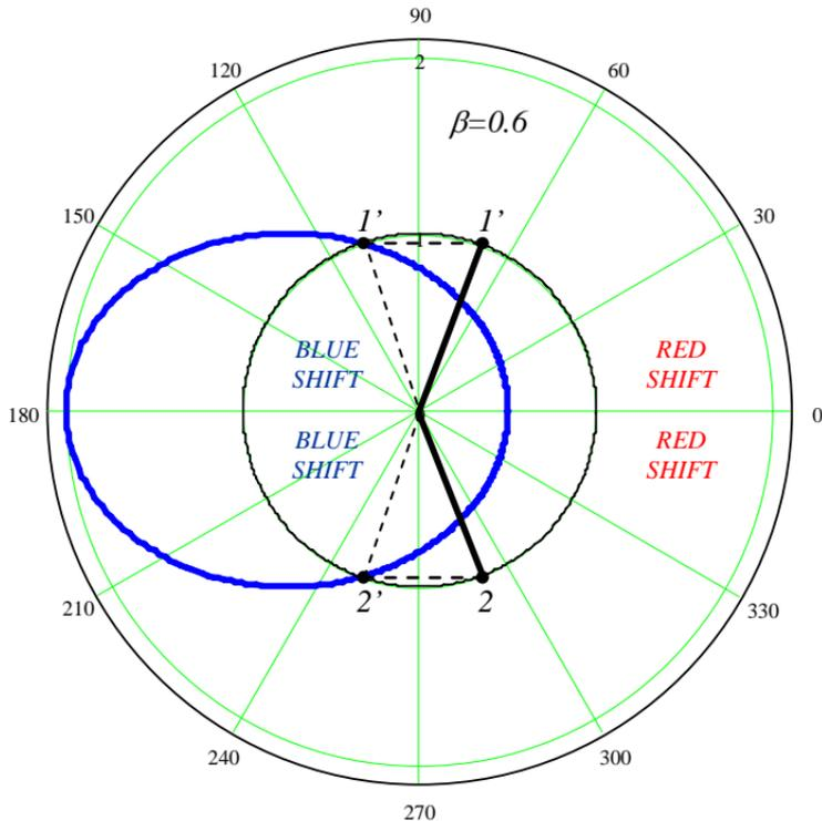
**Figure 11.** Illustrating the directions along which no relativistic effects are detected for radar detection. Separating the regions within which a blue shift or a red shift takes place in the frequency of the electromagnetic radiation.
