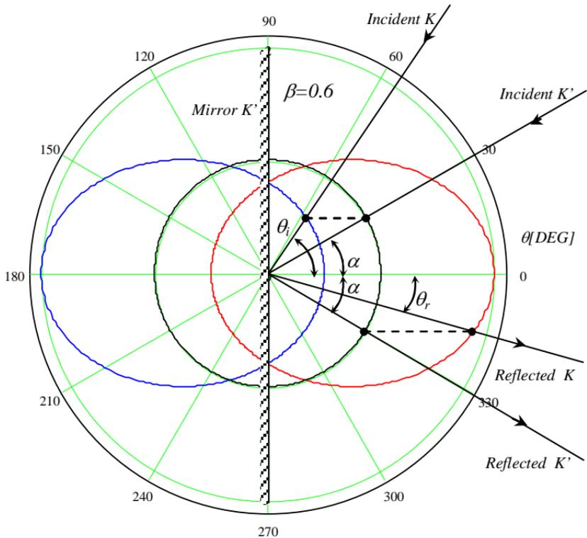
**Figure 10.** Illustrating the way in which observers from  $K$  detect the reflection of light on a vertical mirror at rest in  $K$ .
