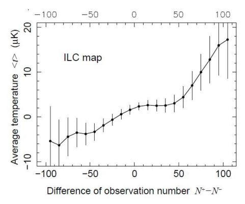
Li et al's figure shows a clear correlation between the temperature calculated by the WMAP team and the difference in the number of times a pixel is observed by the satellite's two antennae.
